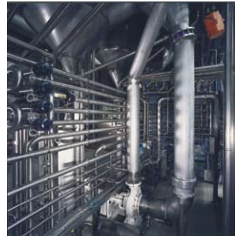
Multi functional evaporator for juices, puree and tomato paste, Italy, type AFV2505S/2-P/To
