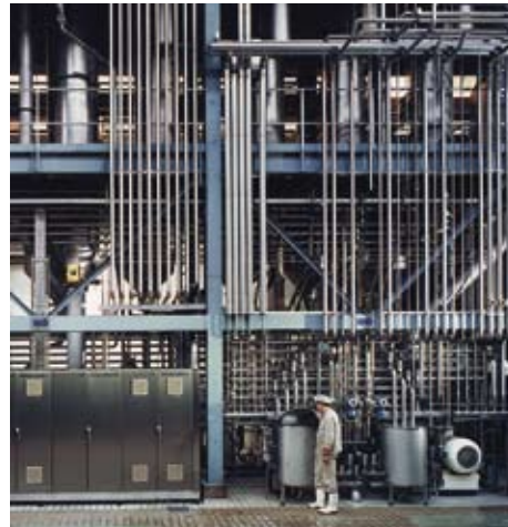
Multi functional evaporator for juices, puree and tomato paste, Italy, type AFV2505S/2-P/To
